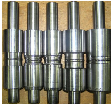
Fig. 4. Thorns on rolling bearing rings
