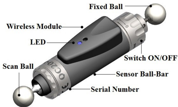
Fig. 2. Sensor Ball-Bar [7]
