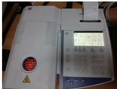
Fig. 3. Moisture analyzer used for measuring straw moisture content before shredding
