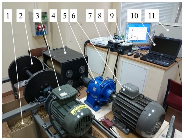
Fig. 1. Research station for the biomass material cutting process: 1 – shredded biomass material, 2 – system of cutters, 3 – electric motor driving rotational movement of the system of cutters, 4 – system of rollers, 5 – reduction drive of the rollers system, 6 – electric motor driving the rollers system, 7 – moisture analyzer, 8 – inverter of the electric motor of the rollers system, 9 – inverter of the electric motor of the cutters system, 10 – PC recording performance of the electric motor of the cutters system, 11 – PC recording performance of the electric motor of the rollers system
