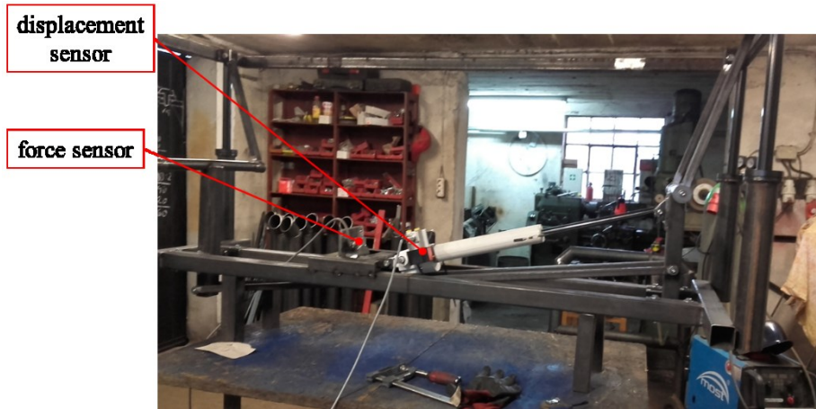
Fig. 9. View of the bed frame when measuring the force needed to power the bed deck height adjustment mechanism
