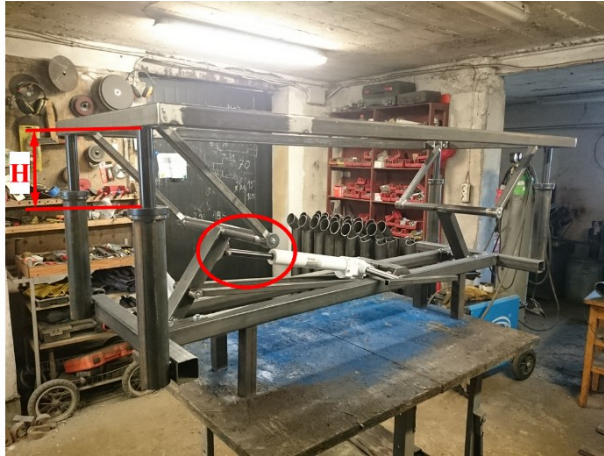
Fig. 7. General view of the bed height adjustment mechanism while in operation – piston rod of the actuator partially extended, bed deck raised to height H
