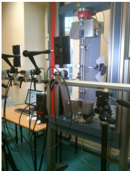
Fig. 6. View of the test stand, bar fixings for the cases considered
