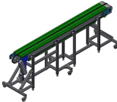
Fig. 1. 3D model of the chain conveyor design
