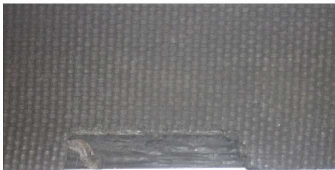
Fig. 6. The friction wear of multi-groove belt
