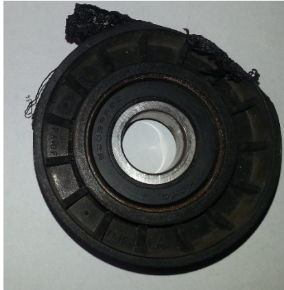
Fig. 13. The sample failure of multi-groove pulley tensioners
