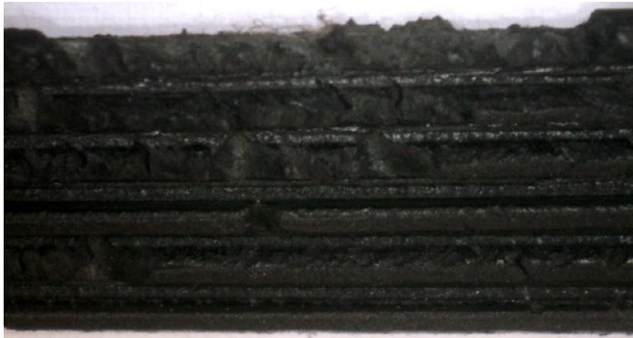
Fig. 7. The damage of the external belt ribs
