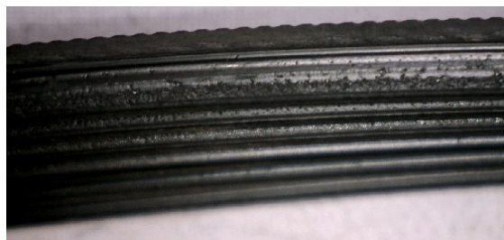
Fig. 5. Peeling phenomenon on multi-groove Belt
