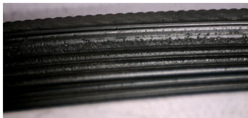
Fig. 11. Fluid contamination in poly-v belts
