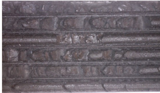
Fig. 4. Rubber flaking in multi-groove belt
