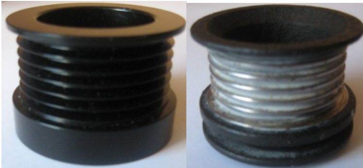
Fig. 12. New pulley and pulley exploited for about 250000 km
