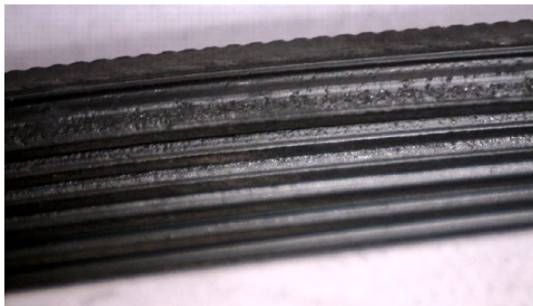
Fig. 8. The uneven wear of the belt ribs
