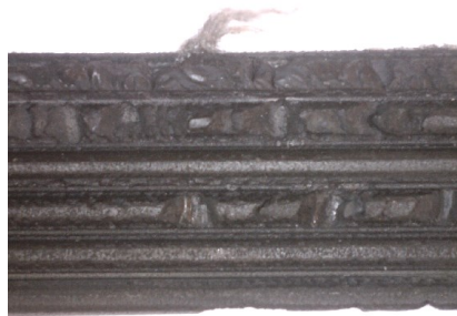
Fig. 10. The band separation
