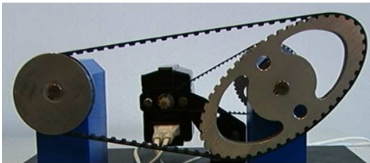
Fig. 2. Two-wheeled uneven-running strand transmission with a cog belt
