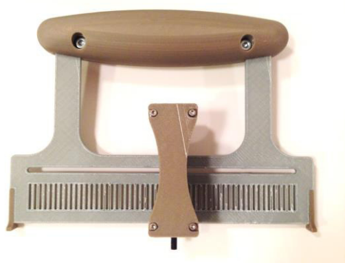
Fig. 2. Visualisation and real view of the handle with sensors
