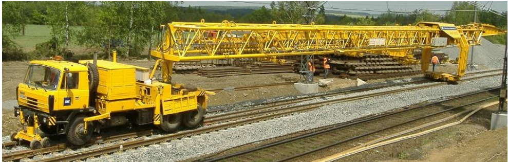
Fig. 5. A Special Railway Crane PKP 25/20i
