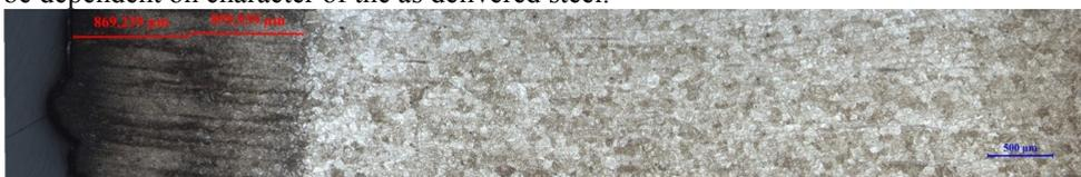
**Fig. 5.** Microstructure under the fracture surface - Toolox 44 – after 50 cycles
