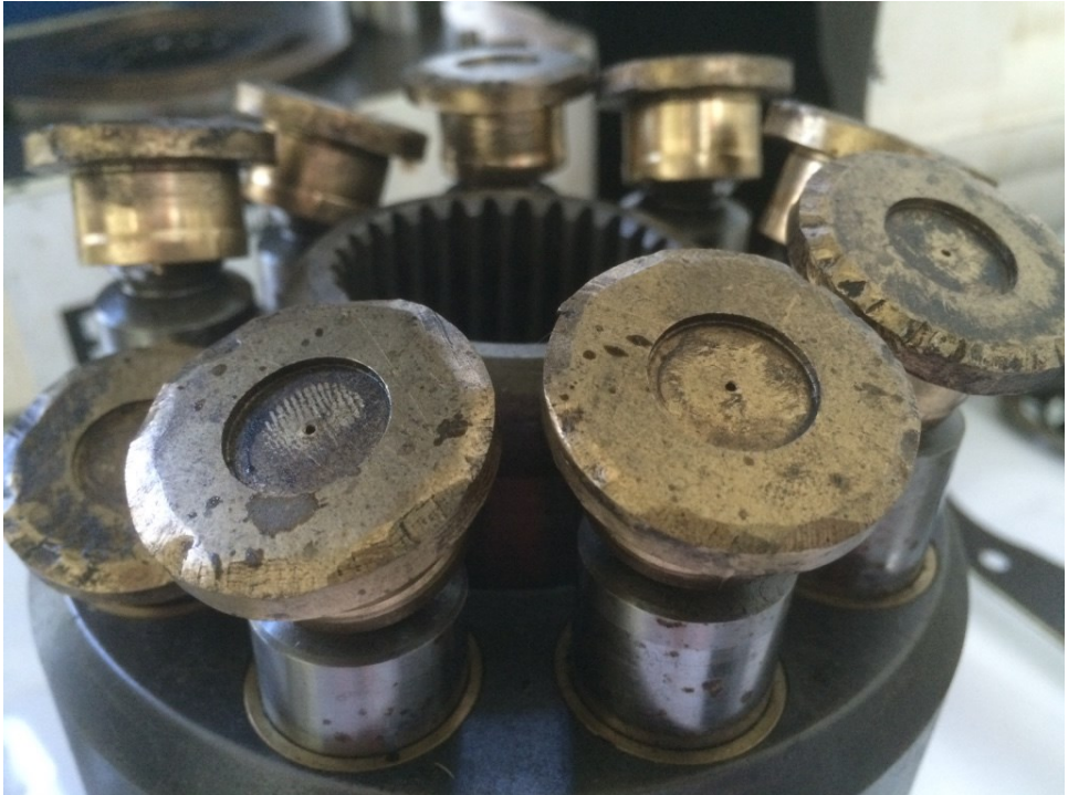
Fig. 5. Hydrostatic slippers of an axial piston pump destroyed due to metal contact with a swash plate surface
