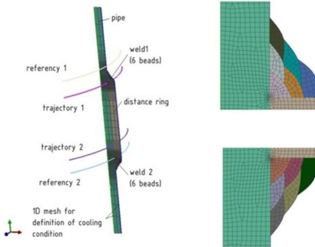
**Fig. 6.** 2D rotational FEM meshed model for simulation
