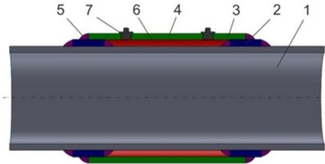
**Fig. 1.** Section of the gas pipeline at repair of gas pipelines with using steel sleeves with composite filling (1 – repairing gas pipelines, 2 – distance rings, 3 – circumferential fillet weld between distance ring and gas pipeline, 4 – steel segmented sleeve, 5 - circumferential fillet weld between distance ring and steel sleeve, 6 – composite filling, 7 – inspection holes) [4]
