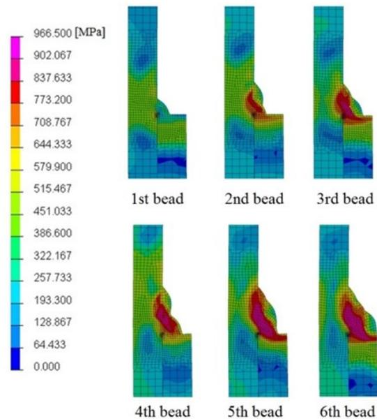
**Fig. 9.** Reduced simulated stresses by Von Misses theory
