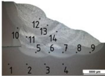
**Fig. 5.** Hardness of weld joint by Vickers
