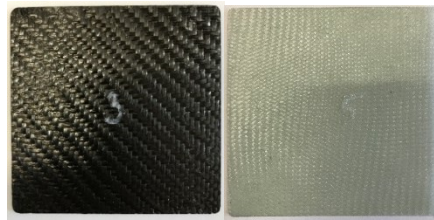
Fig. 2. Laminate with carbon (C#X#) and glass fibres (IGXXX)
