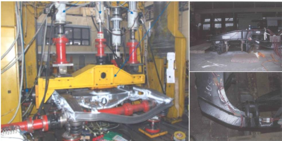
**Fig. 9.** Fatigue and strength tests of prototype bogie frame
