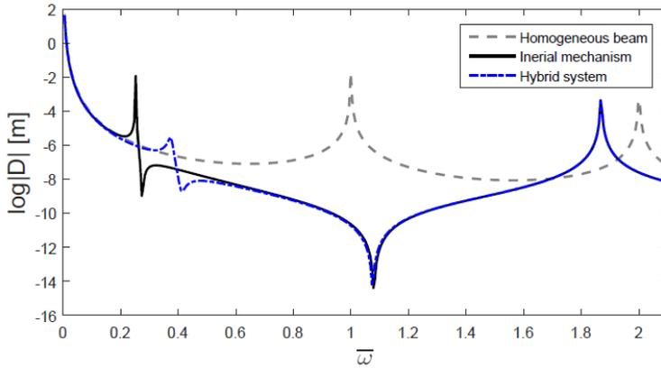
**Fig. 5.** Comparison of the FRF's for different systems
