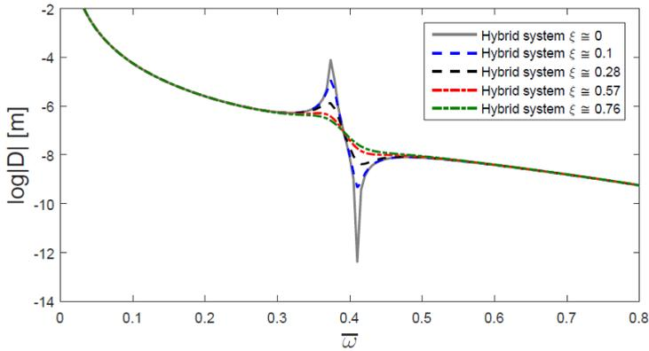
**Fig. 7.** Damping variation of the spring-damper device
