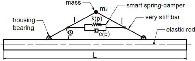
Fig. 2. The elastic rod with attached hybrid mechanism
