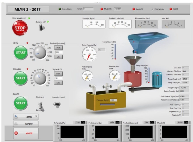
Fig. 2. View of the screen of the control desk of the precise RPW shredder's test stand with measurement of the selected pneumatic transport's parameters
