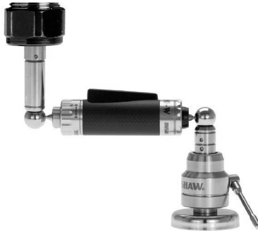
Fig. 2. Renishaw Ballbar QC20-W
