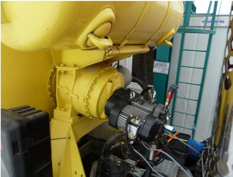
**Fig. 2.** Concrete Transit Mixer Application and prototype of hybrid drive unit
