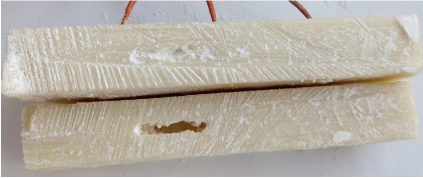
Fig. 3. Shrinkages and cavities in the samples
