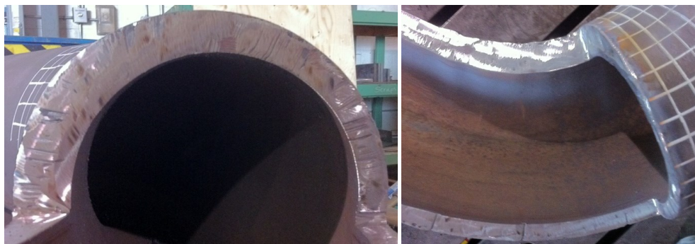
Fig. 7. Final shape of the tube after bending, sectional view of the tube
