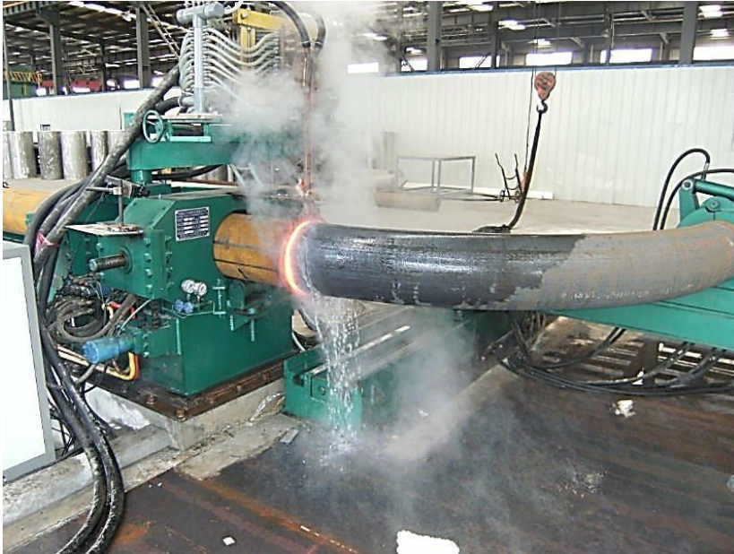
Fig. 2. Device for heat induction tube bending
