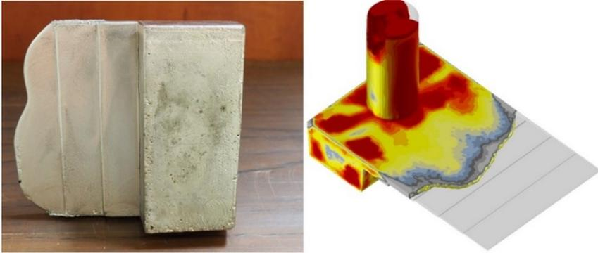
**Fig. 4.** Comparison of casting after completion of the first casting and the first simulation for the first casting design at a mold temperature of 200 °C and a casting temperature of 720 °C
