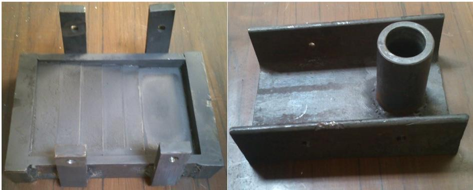
**Fig. 2.** The lower and the upper part of the mold
