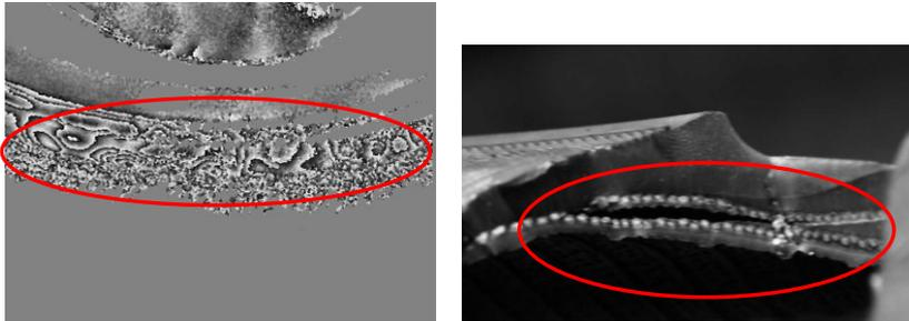
**Fig. 19.** The longitudinal separation in the sidewall of the tyre casing – it is in the site where the carcass lining is bent
