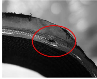
**Fig. 10.** The longitudinal chain separation in the shoulder between the first and second buffer lining
