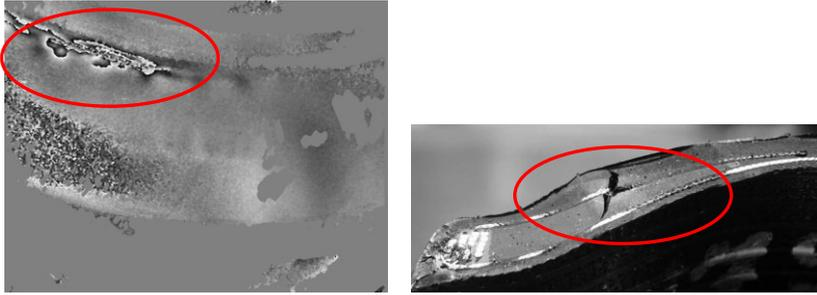
**Fig. 18.** The local separation of the tyre casing - burst bead rubber and bead bundle
