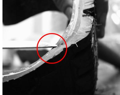
**Fig. 11.** The local separation in the shoulder where the first buffer lining ends
