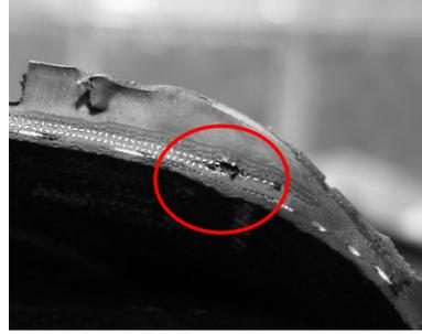
**Fig. 14.** The local separations in the shoulder in the site where the second buffer lining ends
