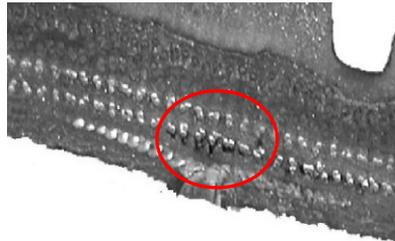
**Fig. 15** The local separations in the crown between the first buffer lining and the cord carcass
