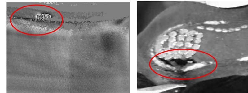
**Fig. 21.** The local separation in the bead area between bead plies and bent - burst bead rubber and bead bundle carcass lining
