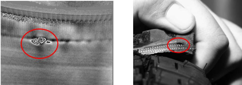
Fig. 8. The local separation in the site where the second buffer lining ends
