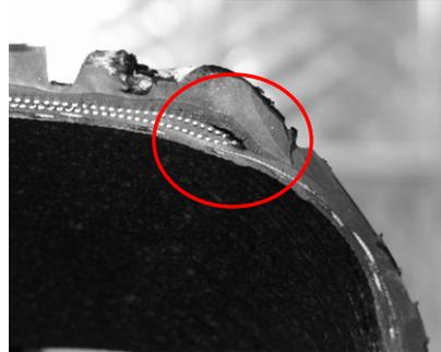
**Fig. 12.** The longitudinal separation in the shoulder where the first and second buffer linings ends and its expanding to the crown
