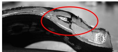
**Fig. 17.** The local separation in the sidewall - burst bead rubber and bead bundle, separation is between the end of carcass lining and bead bundle
