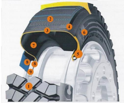
**Fig. 1.** Structure of tyre casing: 1) Tread; 2) Buffer linings; 3) Cord carcass; 4) Filling linings; 5) Bead bundle; 6) Sidewall; 7) Inner skim rubber; 8) Bead reinforcement; 9) Bead plies
