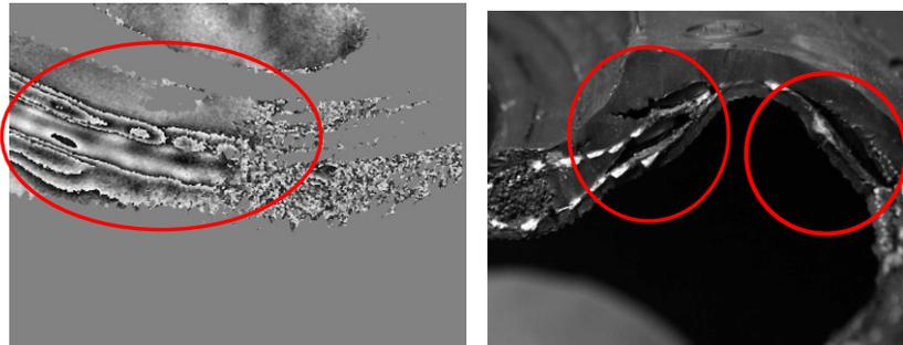
**Fig. 20.** The longitudinal separation in the shoulder and sidewall of the tyre casing between the bent carcass lining and filling linings of bead
