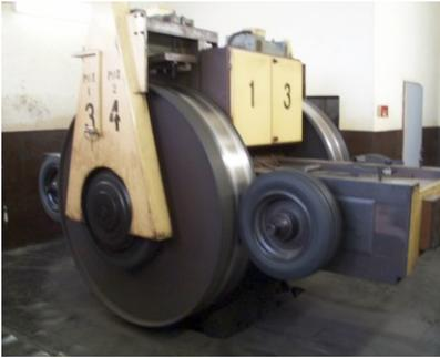
**Fig. 2.** Drum testing device
