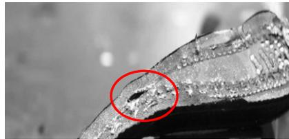
**Fig. 16.** The local separation in the sidewall between the end of carcass lining and bead bundle
