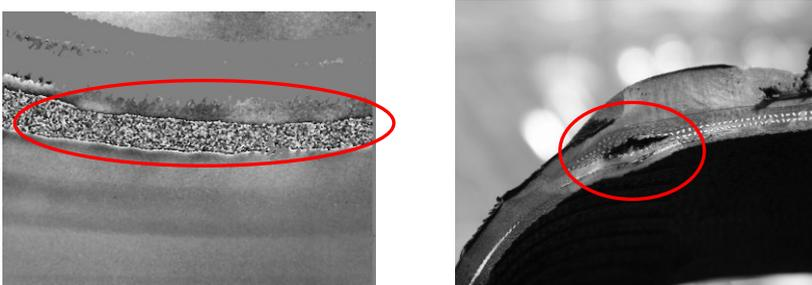
Fig. 9. The longitudinal continuous separation in the shoulder between the first and second buffer lining
