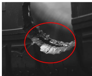
**Fig. 13.** The longitudinal separation in the shoulder and its expansion to the side directions
