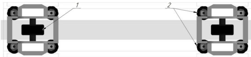
Fig. 2. The scheme of the wheeled vehicle: 1 – traction wheels, 2 – guiding wheels
