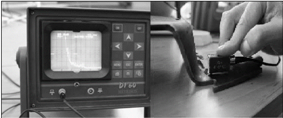
Fig. 12. Defectoscopic examination of 8 samples - no cracks
