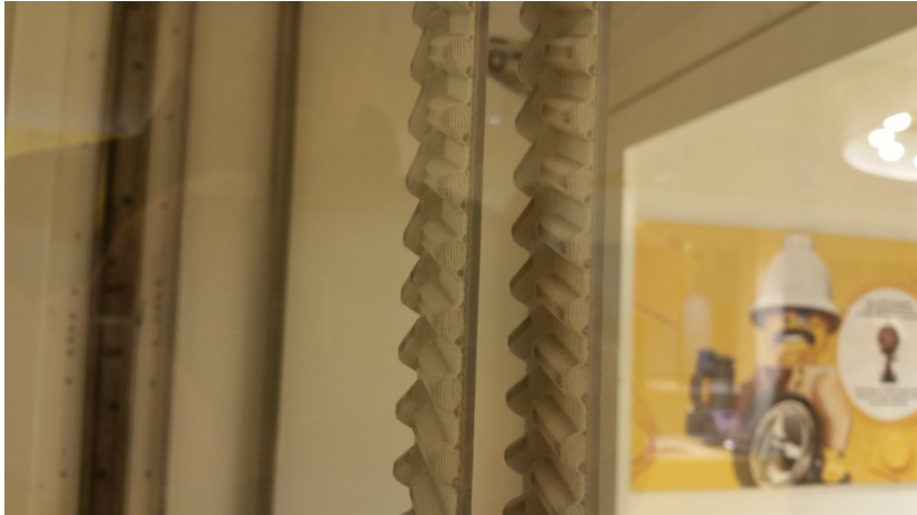
Fig. 2. Herringbone toothed belts in a passenger lift
