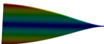
Fig. 17. Modal torsional shape at natural frequency 125.2 Hz, FEA ANSYS, No. 2, a side view, the shape not detected by the IR camera
