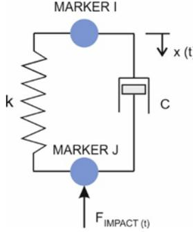
**Fig. 3.** Model of unilaterial impact force by the IMPACT function
