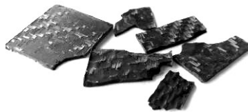
Fig. 8. The rest of the glue with the teared fibers from carbon fiber laminate
