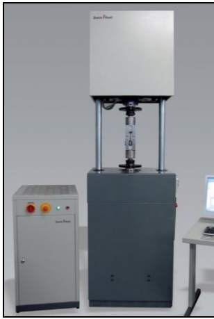
a) fatigue experimental machine Zwick/Roell Amsler 150HFP 5100
